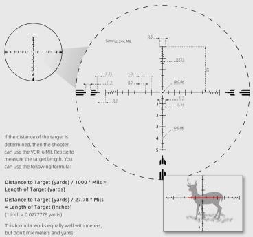
Distance to Target(meters) / 1000 \* Mils = Length of Target (meters)
