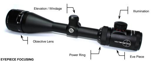
The eyepiece is designed to provide a precise fast focus (remove the flip-up cap if covered on ocular lens). The eyepiece will focus faster than your eye can compensate for any inaccuracy in your adjustment.
